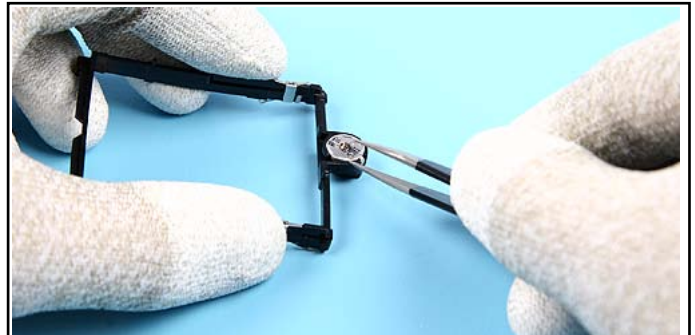
26. Note the grounding clips of the DISPLAY FRAME ASSEMBLY when removing the EARPIECE.
