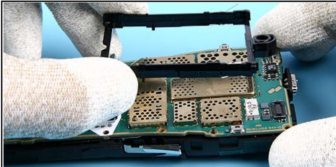
25. Remove the DISPLAY FRAME ASSEMBLY.
