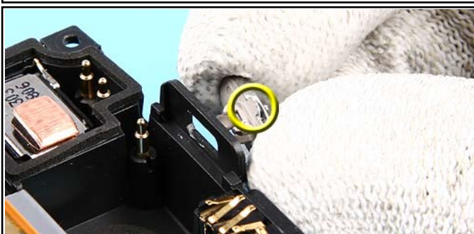
15. Mind the correct position when placing the HOLD SWITCH HANDLE.
