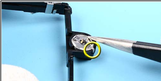
29. Place the Earpiece into the Display Frame Assy. Do not bend the grounding clips. Mind the guiding pin of the EARPIECE.
