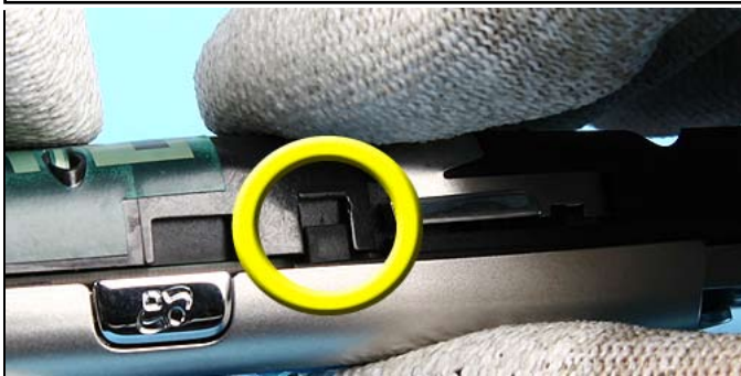
45. Note that both clips are locked properly.
