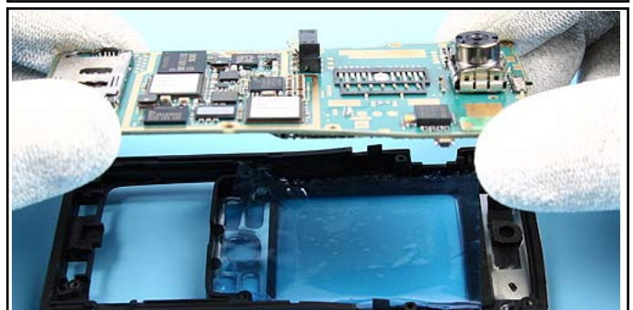
32. Use an A-COVER as support when removing the CAMERA MODULE.
