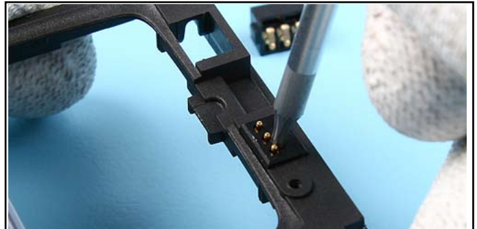
18. Push out both SLIDE CONNECTOR POGOs .
