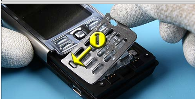
47. Place the BEZEL COVER at the shown side first.
