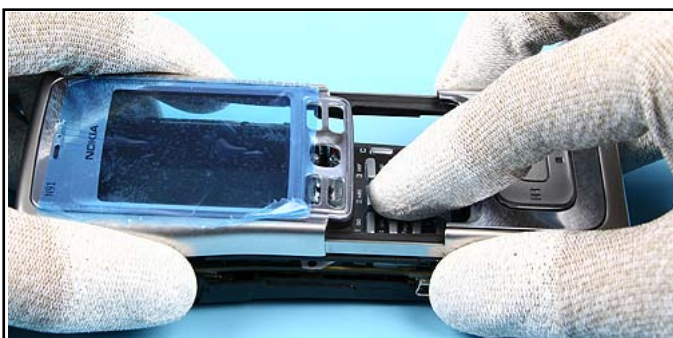
10. Push down the KEYMAT while lifting of the SLIDE ASSEMBLY.
