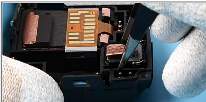
11. Place the IHF SPEAKER. Always use a new IHF SPEAKER GASKET when replacing the speaker.
