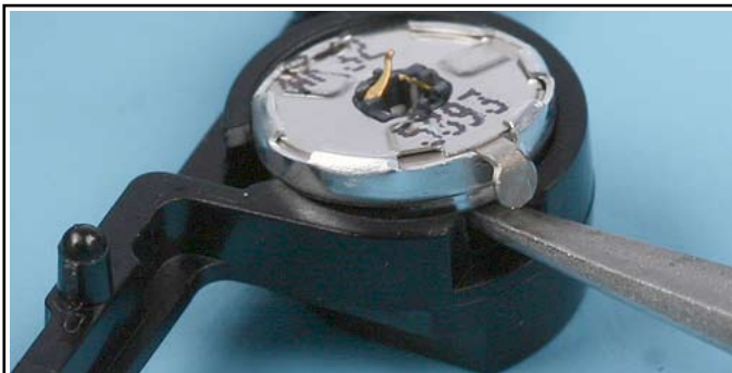
27. Lift up and remove the EARPIECE with tweezers carefully.
