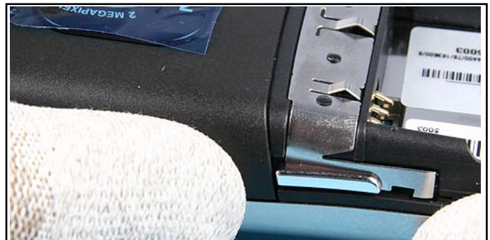
54. Note the correct positioning of the ANTENNA COVER ASSEMBLY.
