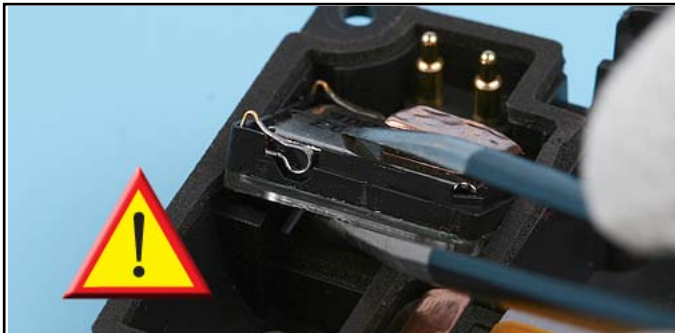
41. Carefully remove the IHF SPEAKER. Do not touch the membrane.
