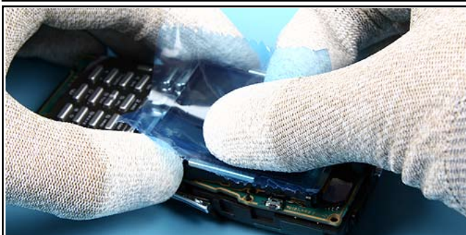
12. Protect the LCD with a plastic film, too.
