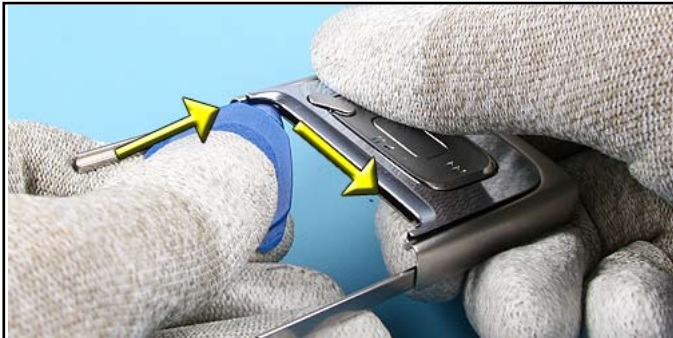
19. Carefully release the adhered SLIDE BEZEL as shown.
