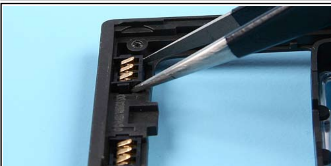
36. Insert the two SLIDE CONNECTOR POGOs.
