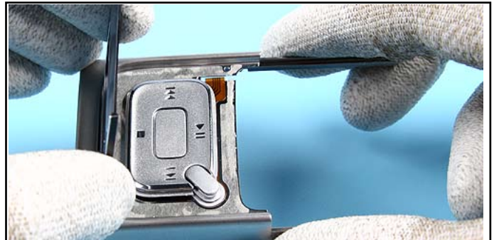
20. Remove the SLIDE BEZEL carefully.
