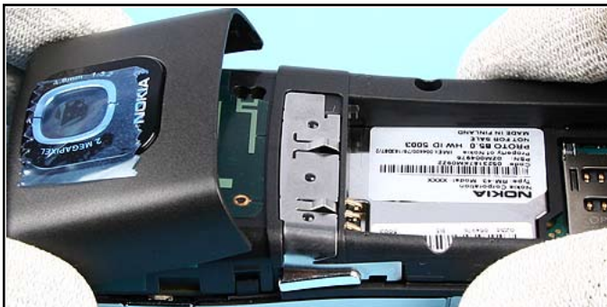
53. Place the ANTENNA COVER ASSEMBLY beginning from the top.
