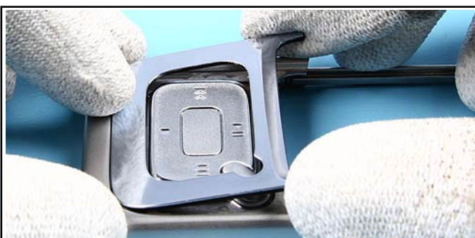
34. Always use a new adhesive when fitting the SLIDE BEZEL.
