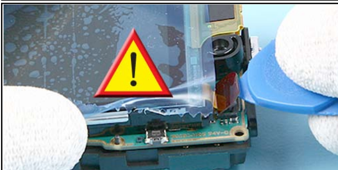
23. Open the LCD flex connector.
