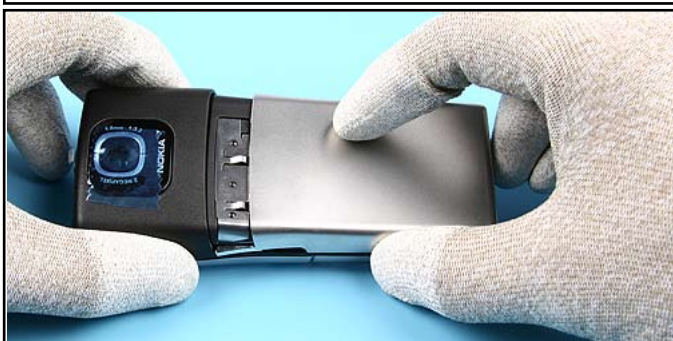
55. Assemble the B-COVER ASSEMBLY.
