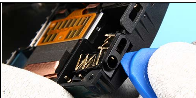
38. Lift the 3,5 AUDIO JACK and remove it.
